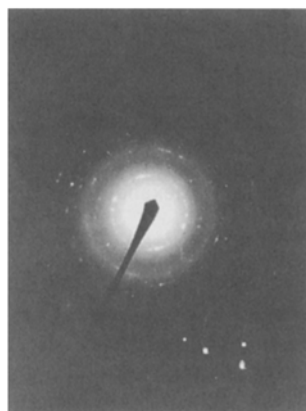
Fig.4 Electron diffraction image of the nanocomposite shown in Fig.3
